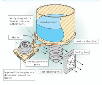
The new detector and new unique furnace construction achieves a noise level of less than  $0.5\mu W$ , ensuring a stable baseline.
