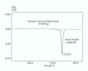
A stable baseline and S/N performance enable the detection of a minute calorimetric change during trace analysis.
