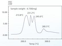
Measurement of Battery Material (LiB. Active material)
